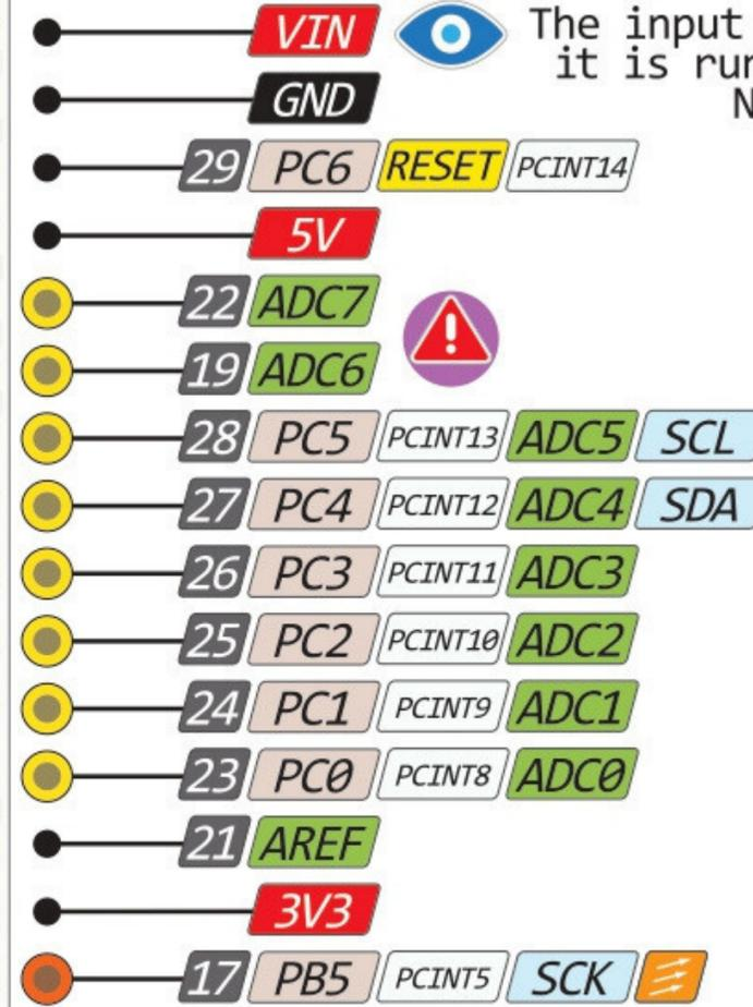
The input voltage to the board when it is running from external power. Not USB bus power.
