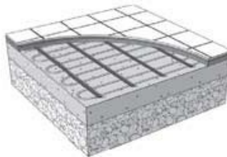
MA ICE-30 cable under tile
