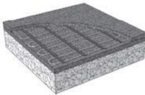
MA ICE-30 cable in asphalt
