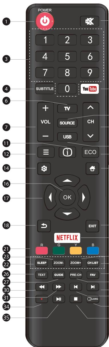
1. : Switch the TV between on and standby mode
