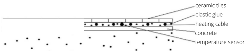
Figure 2: Directly on the concrete
