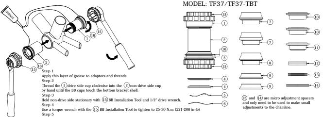
Install any necessary adaptor, according to chart.
