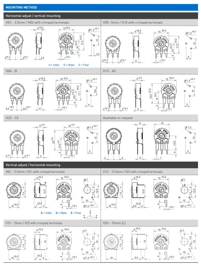
15-mm carbon / cermet through-hole potentiometer
