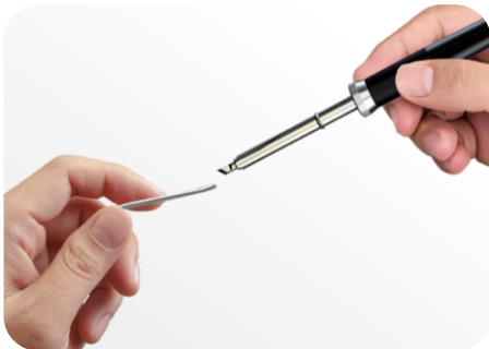
3 Clad The lifespan of the soldering tip can be prolonged by cleaning it with tin.
